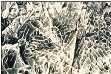
Figure 1. Microstructure of etched porcelain.
